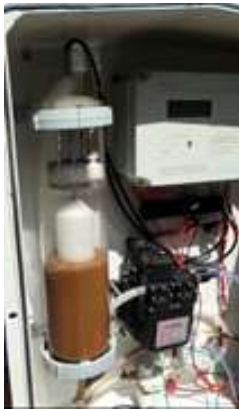
Silt sample is filled inside the sampling tank Just before measurement
