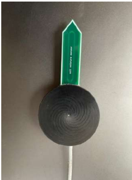
Soil Wetness + Soil Temperature sensor: (Capacitance type)
