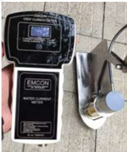
Suspension type water current meter with hand held display unit
