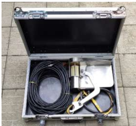
Suspension type Current meter for river gauging.
