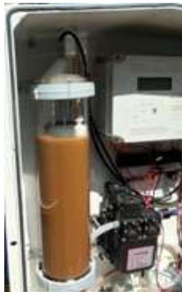
Silt sample is filled inside the sampling tank Just before measurement
