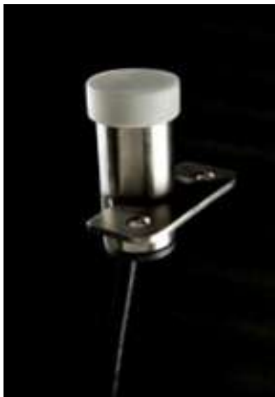
Solar Radiation sensor
