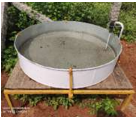
Capacitance type Evaporation sensor
