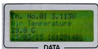
Size of the new Dot Matrix digital display: Total size of the display: 76 x 25 mm.
